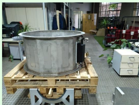
Figure 20: decagonal WHRU system
